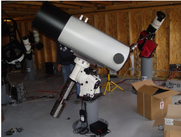
ISON-NM: SANTEL-400AN, D=400 mm, f/3, FOV 106'x106' CCD – FLI ML09000-65
